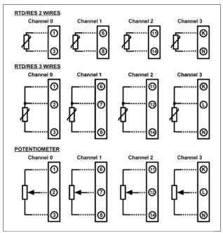
Terminals 3,8,14, and N = input negative reference. Terminals 13 and M not connected (NC).
