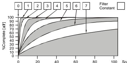
0 20 40 60 80 100 Scans **Digital Filtering.** The illustration above demonstrates the effect of digital filtering (set with Filter Constant) on module response to a temperature change.
